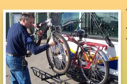
move the support arm out of the way Lift your bike out of the rack Always fold up the bike rack if there is
