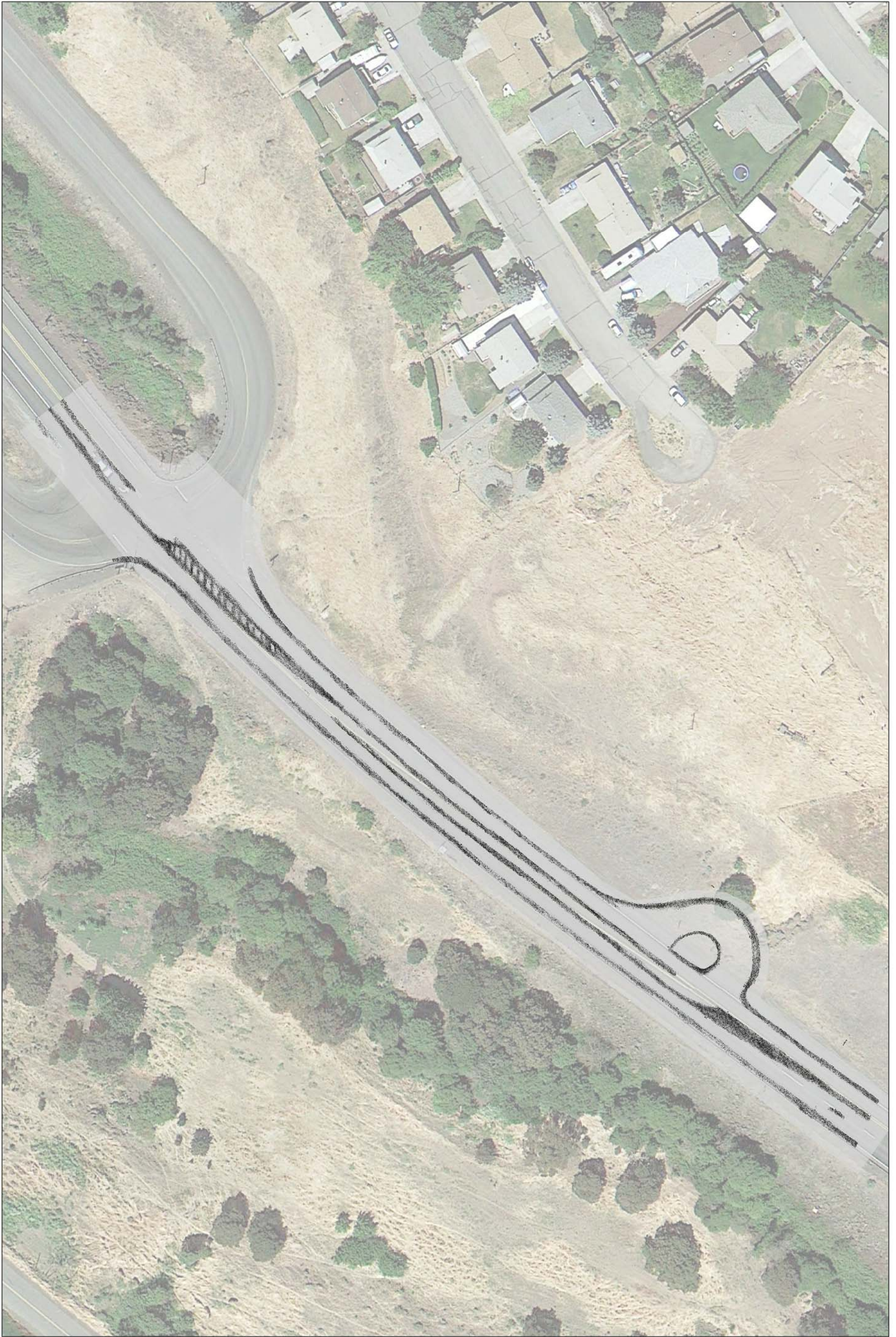
PROJECT I-2: CONCEPTUAL J-TURN ALTERNATIVE US 197/FREMONT ST/COLUMBIA VIEW DR THE DALLES, OR
