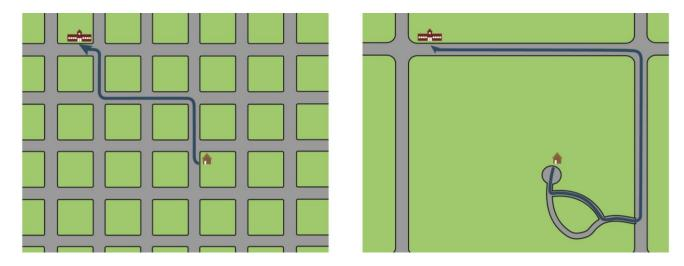
The left illustration is a connected street grid, on the right is a less connected system. Travel distance from home to school is shorter in a connected system.
