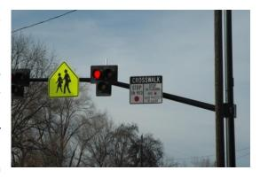
some cases, at unsignalized intersections (the MUTCD suggests that the beacons be located at least 100-feet from an intersection). Pedestrian Hybrid Beacons could be used at any unsignalized intersection or mid-block crossing where warrants require a higher level of crosswalk protection.
