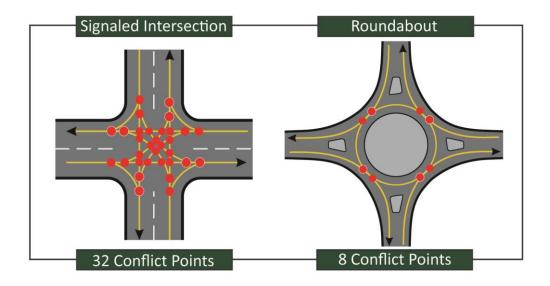
Depending on the design, roundabouts can be more land-intensive than other intersection controls. To maintain the flexibility to construct roundabouts at key intersections, the City may want to ensure adequate right-of-way is provided at intersection locations whenever right-of-way dedication or acquisition activities are undertaken. Information contained in the City's development code and engineering standards can account for this need.
