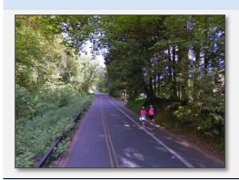
A mixed-use shoulder is a roadway shoulder that is wide enough to be used by pedestrians and bicyclists as a mixed-use path. Mixed-use shoulders are ideal on low-volume streets where topography or the surrounding environment does not allow for the addition of a sidewalk or separate bicycle facility.
