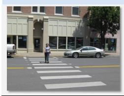
Clear, reflective roadway markings and accompanying devices are placed at intersections and priority pedestrian crossings where there is sufficient sight distance and reaction time for motorists to yield. Crosswalks can be used at intersections and at midblock crossings.
