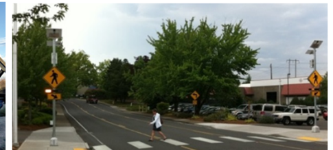
Rectangular Rapid Flashing Beacons
