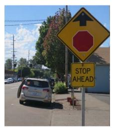
This STOP AHEAD sign, located on Ridgegate east of Oatfield, should be on a separate signpost. The City should consider moving the STOP AHEAD sign closer to the STOP sign to which it applies, and replacing it with a Stop Ahead symbol sign.
