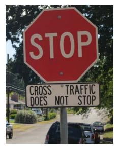
When this STOP sign plaque is replaced for maintenance reasons, the new plaque should be black and yellow.
