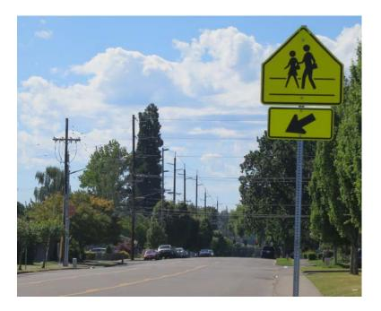
This school crosswalk sign with the diagonal arrow is properly located, but is an older-style sign with crosswalk lines on the sign. When this sign needs to be replaced for maintenance reasons, the current standard (without the crosswalk lines on the sign) should be used.
