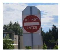
This DO NOT ENTER sign at the Gladstone High School exit driveway obscures much of the STOP sign. The DO NOT ENTER sign could be mounted lower on the post or on a separate post.
