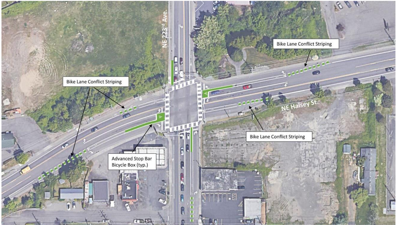
Figure 3: Near-term Intersection Treatments – NE 223 rd Avenue
