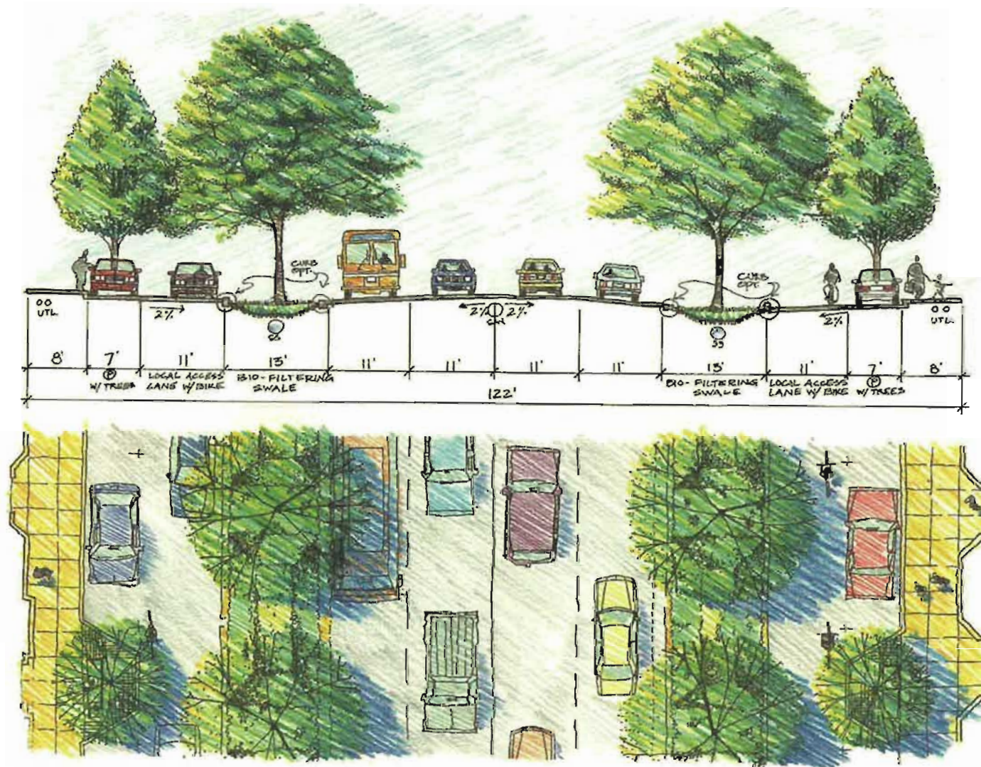
Figure 6-2 Double Median Boulevard with Bio-Filtering Swales
