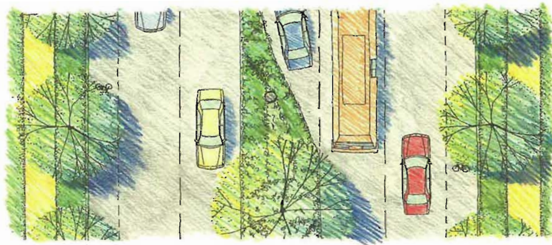
Figure 6-5 Regional Street with Median Bio-Filtering Swale
